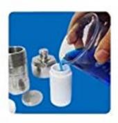
Pour reaction material into PTFE / PPL liner.
