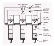
Fig. A: Initial state. Manifold pressure builds to controller set pressure. The effect of the restrictors is minimal in limiting flow from manifold to column reservoir. Reservoirs start at Atmospheric pressure.
