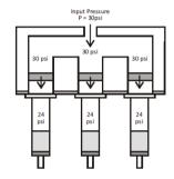
Fig. C: Depending on flow characteristics of column sorbent bed, pressure in column reservoir stabilizes...
