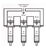
Fig. B: Shortly after the initial state, the pressure builds in the column reservoir due to the fluid being held up by the flow characteristics of the column sorbent bed. Restriction still has minimal effect. Eventually the pressure builds enough to overcome the fluid flow resistance and the fluid begins to pass through the sorbent bed.
