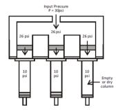
Fig. D: When fluid passes through (one or more columns) completely, and there is minimal pressure drop across the column bed, the effect of the restrictor is maximized. The restrictor becomes the primary flow inhibitor of the gas as it passes through the column to the atmosphere.
